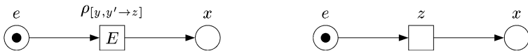
Fig. 12. Operator net for E[y, y' \rightarrow z] , and Petri net for constant z .
